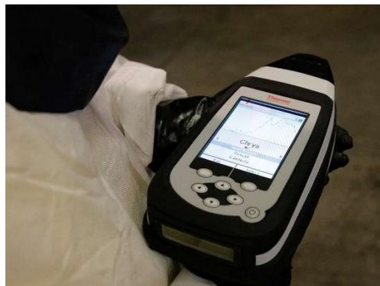
*Thermo Scientific's microPHAZIR AS can provide ACM identification in seconds*
